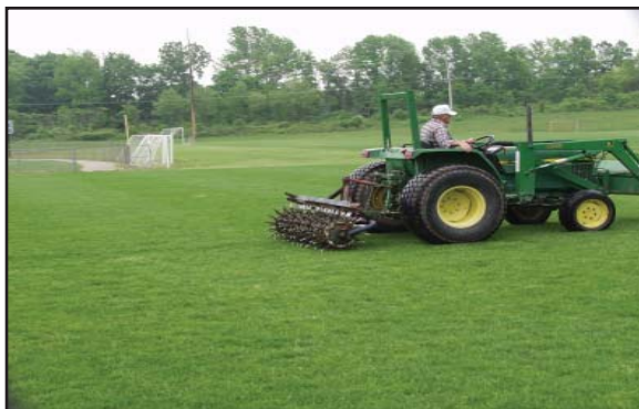
Figure 4. Aerifying a lawn helps reduce thatch and increase water movement when tine size and spacing is adequate (Z. Reicher).
